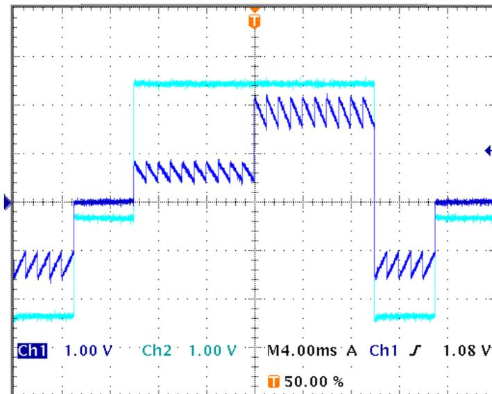
Figure 7 : Bi-level Ramped Pulse
